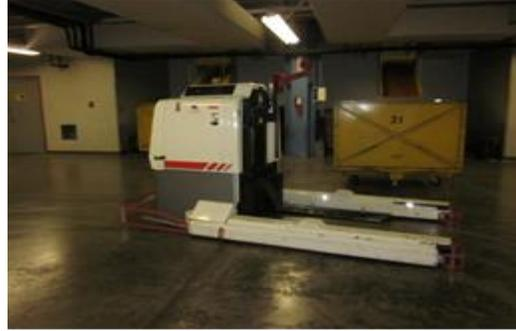
*This “robot” machine picks up and moves the 2000-pound rolls of paper so that there is no human materials handling risk exposure.*
